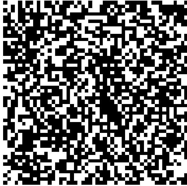
Fig.5. Site percolation on a grid 50 \times 50 . Probability of a site being occupied is equal to the critical concentration p_c = 0.5899 .
